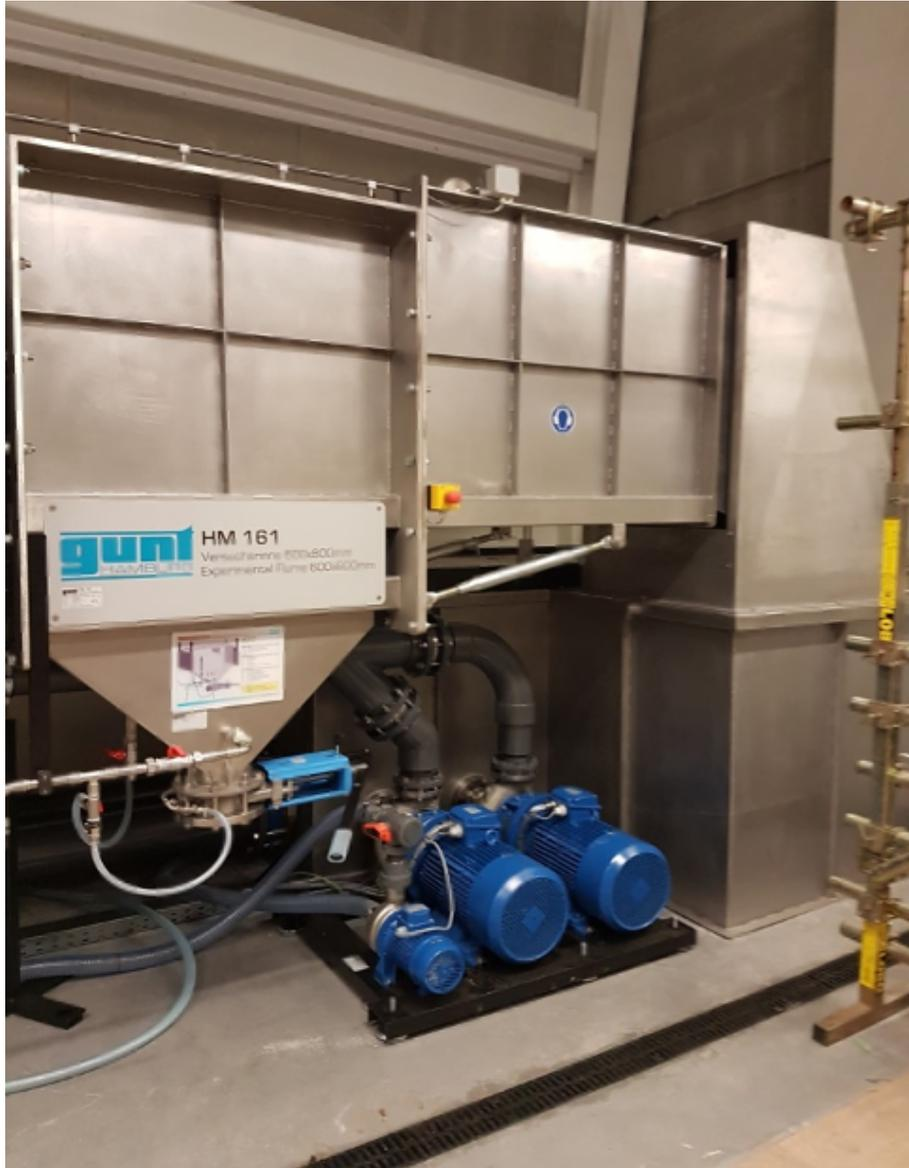
Figure 2: Centrifugal pumps used to recirculate water in the flume. Notice that the small pump on the left is used to recirculate sediment, and was not used in the experiments described in this report.
