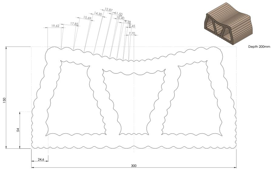
Figure 6: CAD model of the prototype-scale brick.
