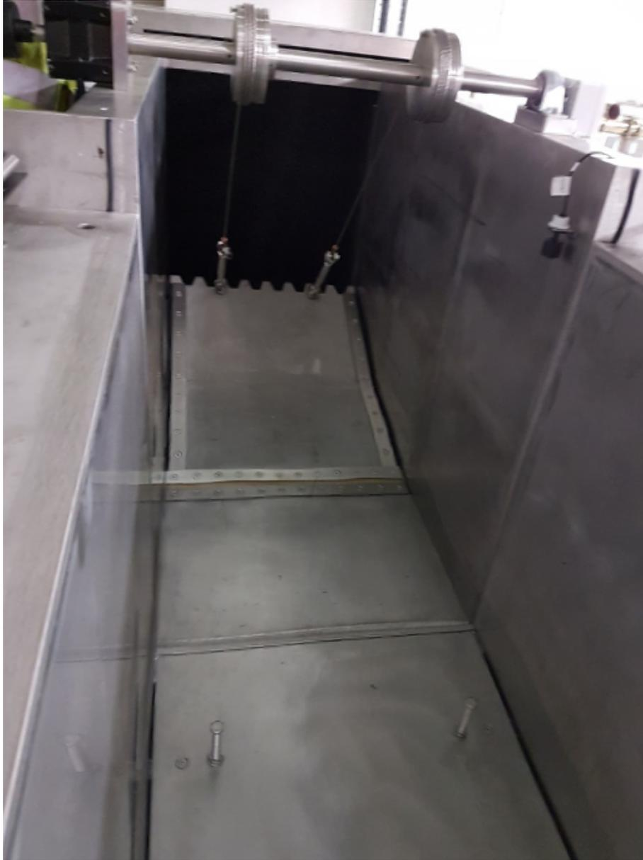
Figure 4: Downstream gate used to control the water surface elevation in the flume.
