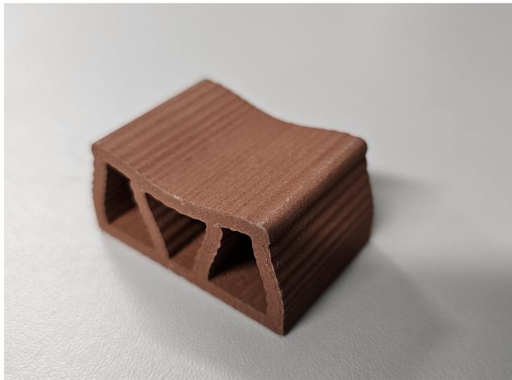
Figure 7: Photo of the 3D-printed brick.
