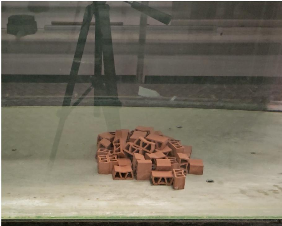
Figure 10: Distribution of bricks in Test 4.
