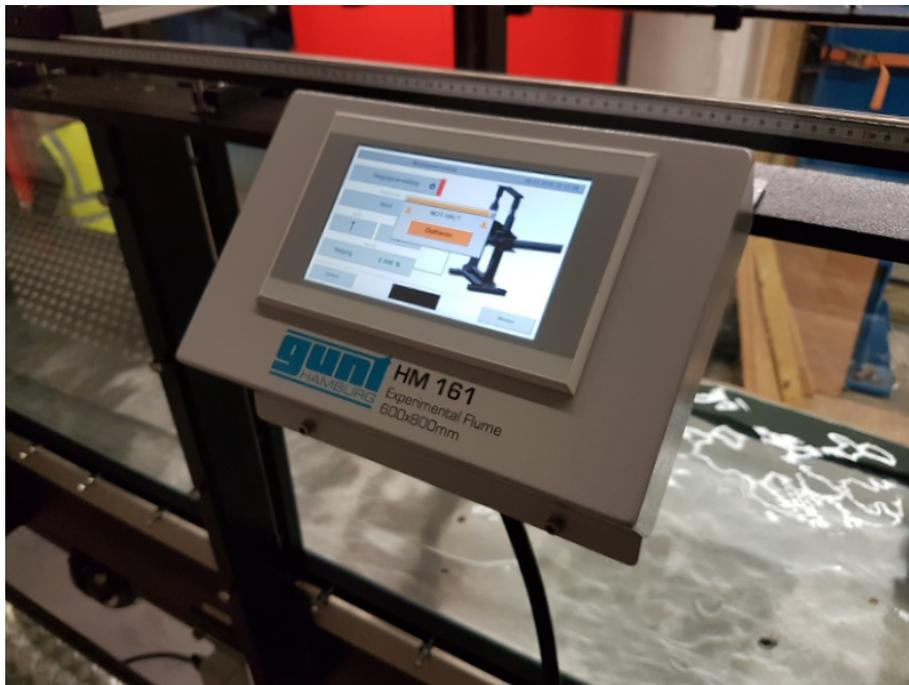
Figure 3: Control panel used to set the flume's slope and the flow discharge.
