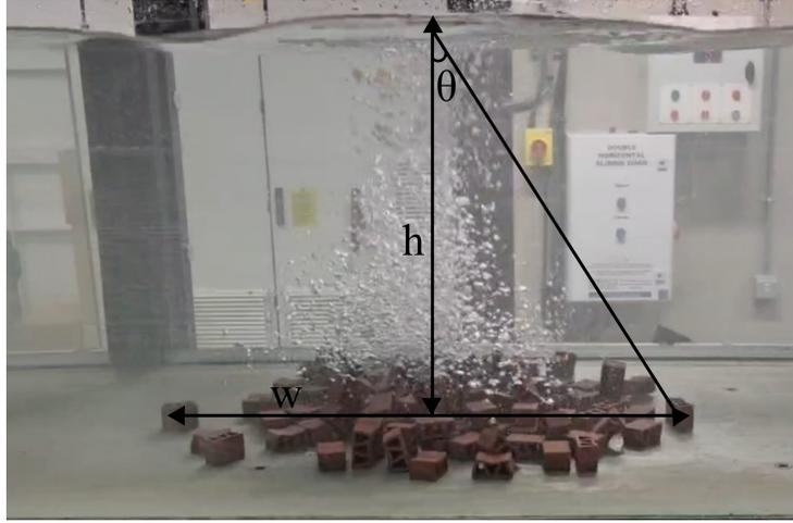
Figure 12: Photo of the spread of the bricks.  $w$  is the width of the spread area,  $h$  is the water depth and  $\theta$  is the spread angle.
