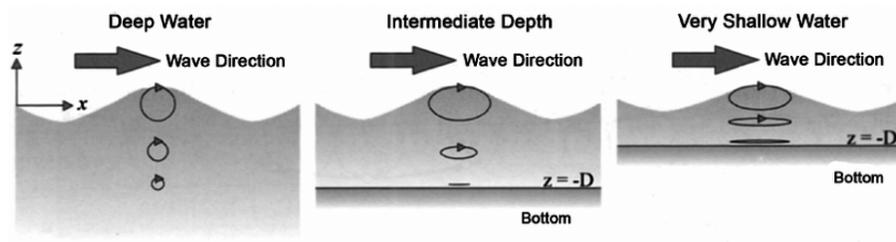
Figure 13: Particle motion in waves
