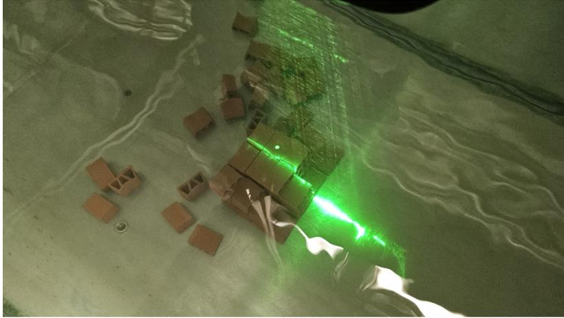
Figure 5: The sampling plane illuminated by a laser sheet.
